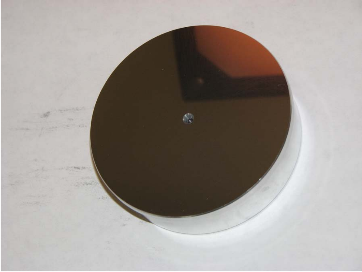
Nice surface This was done on a 1800 mesh Ablap in a few minutes.
