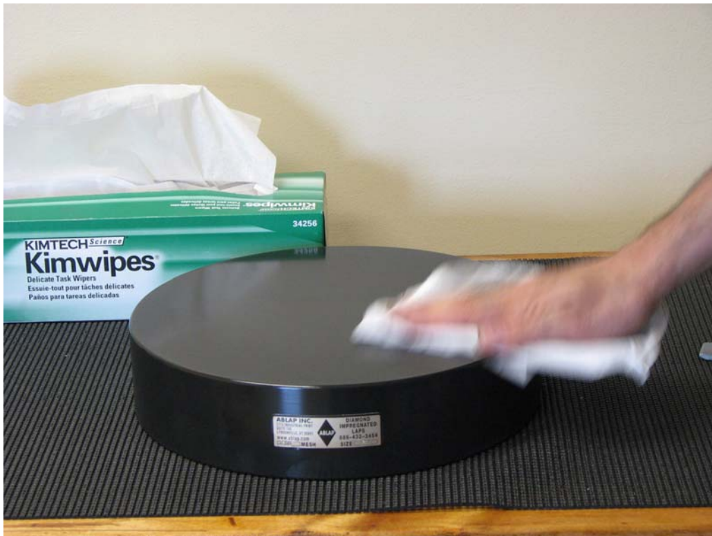
Spread lube over Ablap and wipe off excess. Too much oil will cause parts to float on surface.
