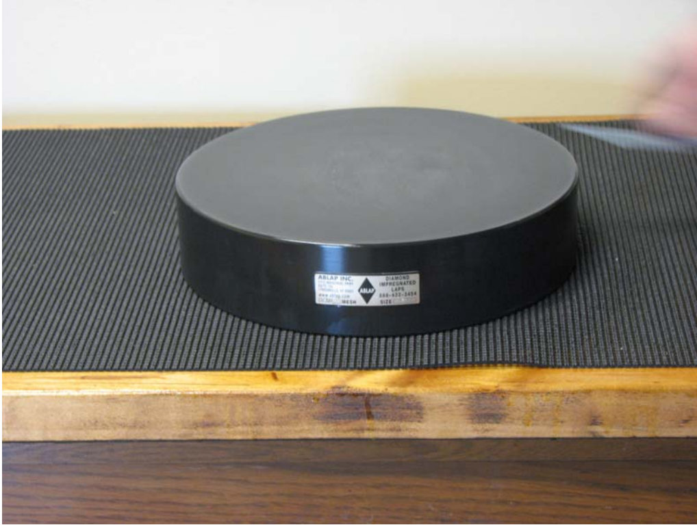
The cleaning stone has been applied over the entire surface.
